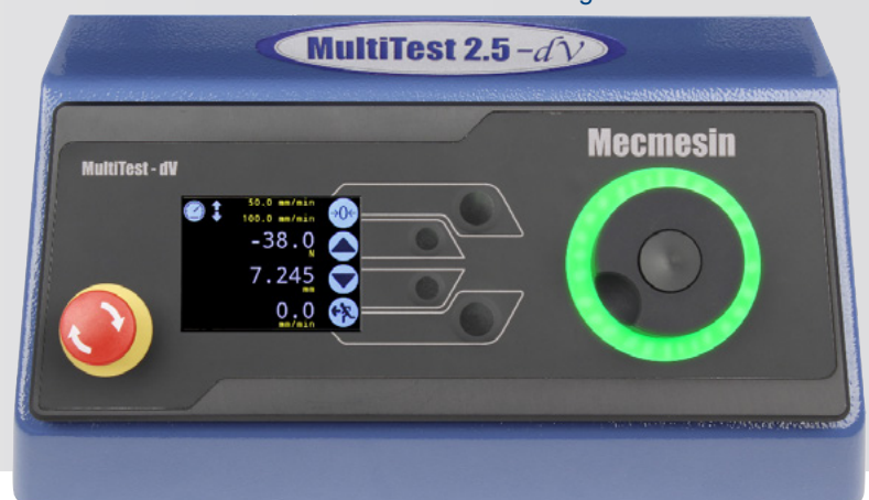
▲ Lights indicate stand status Dial positions crosshead precisely Centre button confirms menu settings
